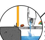
**Bunded** non slip concrete floor to contain 25% of total volume or 100% of the largest package
